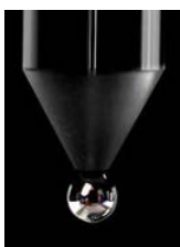
Figure 9. A dropping mercury electrode (from Bioanalytical Systems, Inc, 2012).
