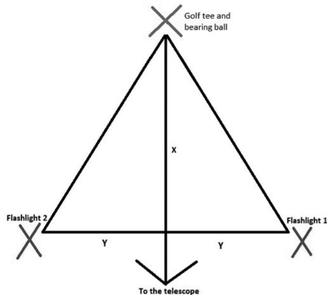
**Figure 2: Artificial double star arrangement to calibrate the filar micrometer.** The  $x$  and  $y$  parameters are changed depending on the desired separation. The flashlights used are directed toward the bearing ball in this arrangement. The bearing ball then reflects the light from the flashlights to the observer at the telescope.
