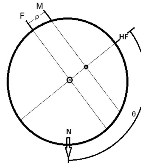
**Figure 1: Measuring double stars with a filar micrometer.** HF is the horizontal fixed wire of the filar micrometer. F is the vertical fixed wire. M is the vertical moveable wire. N is north in the field of view.  $\theta$  represents the position angle of the double star.  $q$  represents the separation of the double star. The primary star is at the intersection of F and HF. The component star is at the intersection of M and HF.
