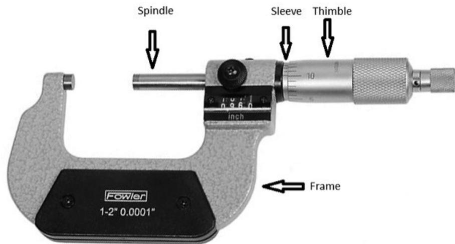
**Figure 4: The Fowler 1-2” digital micrometer.** The spindle remains in contact with the slide and enables measurement of the location of the moveable wire. The sleeve increases the precision of the micrometer to the ten thousandth of an inch. The thimble is rotated to move the spindle linearly. The frame fits into the slide casing which keeps it in a consistent location.
