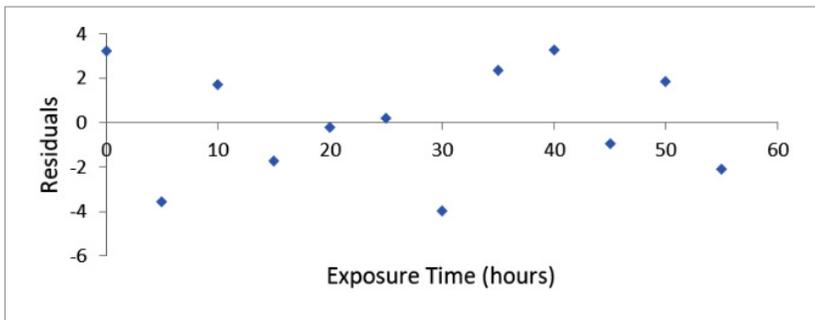
**Figure 3: Plot of residuals vs the time submerged in FLiNaK molten salt.** The residuals show the deviation of each average hardness value from the expected values calculated by the regression analysis, which means that ideal linear data would lie entirely on the x-axis. The exposure time is the duration that the Hastelloy N sample was submerged in the molten FLiNaK salt.
