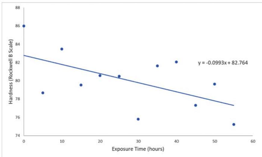
**Figure 2: Hastelloy N samples hardness decrease upon increasing exposure to FLiNaK.** The hardness values displayed on this plot are the average of twenty hardness readings from each of the fourteen Hastelloy N samples. A linear trend line fitted to this data is shown along with its representative equation.
