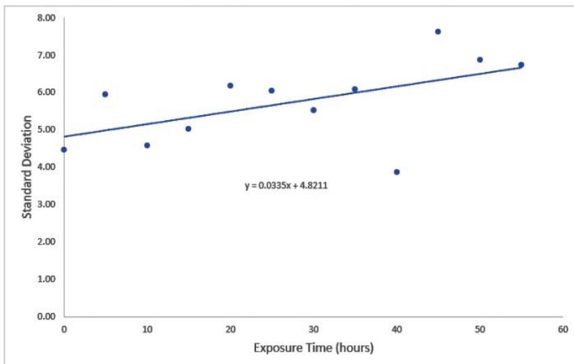
**Figure 4: Standard deviation in hardness increases upon increasing exposure time.** The standard deviation displayed on this plot are based on the twenty hardness readings from each of the fourteen Hastelloy N samples. The exposure time is the time that the sample corresponding to each standard deviation value was submerged in the FLiNaK molten salt. A linear trend line fitted to this data is shown along with its representative equation.
