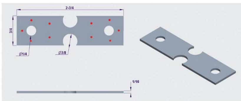
**Figure 1: Dimensions (in inches) of machined Hastelloy N samples.** These dimensions are based on measurements of an existing sample used for testing on the Rockwell Hardness Tester used in this study. The dots in the figure represent the approximate location that the hardness was tested (ten on both sides of the sample).
