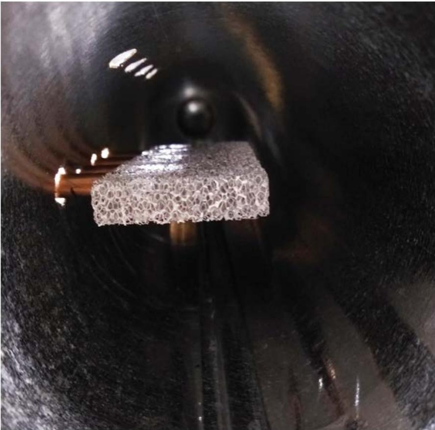
**Figure 6: Heat pipe and aluminum foam positioning.** The aluminum foam and heat pipes are inserted similarly to the initial test with only heat pipes. The test conducted with aluminum fins was identical as well.
