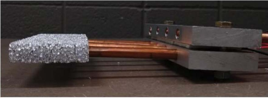
**Figure 5: Aluminum foam positioning.** The heat pipes are inserted into the aluminum foam block.
