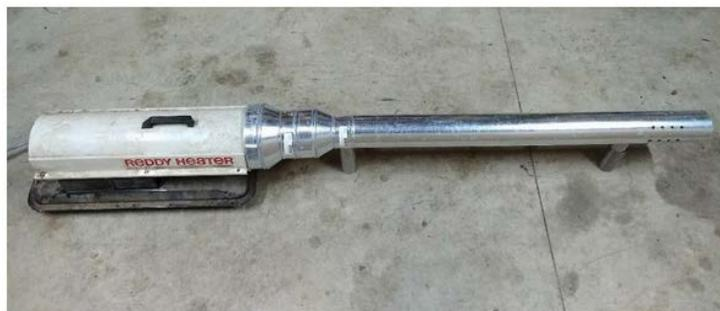
**Figure 1: Automotive exhaust heat simulation device.** A forced air kerosene heater coupled with metal duct was used to simulate an automotive exhaust system.
