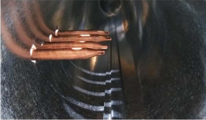
**Figure 2: Heat pipe positioning in duct.** Four heat pipes were separated by a distance of 30 mm and inserted 76 mm into the metal duct.
