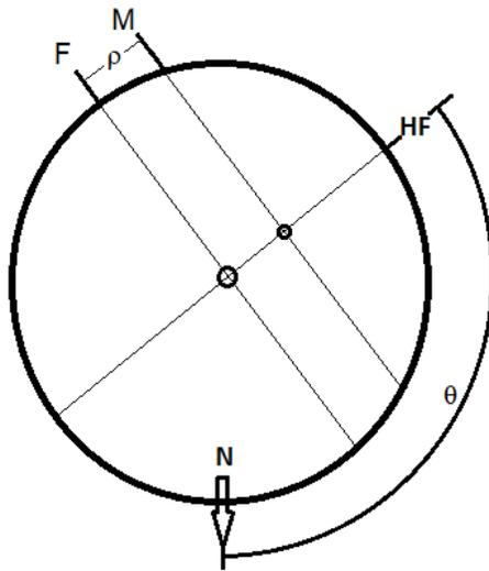
**Figure 1: Measuring double stars with a filar micrometer.** HF is the horizontal fixed wire of the filar micrometer. F is the vertical fixed wire. M is the vertical moveable wire. N is north in the field of view.  $\theta$  represents the position angle of the double star.  $\rho$  represents the separation of the double star. The primary star is at the intersection of F and HF. The component star is at the intersection of M and HF.
