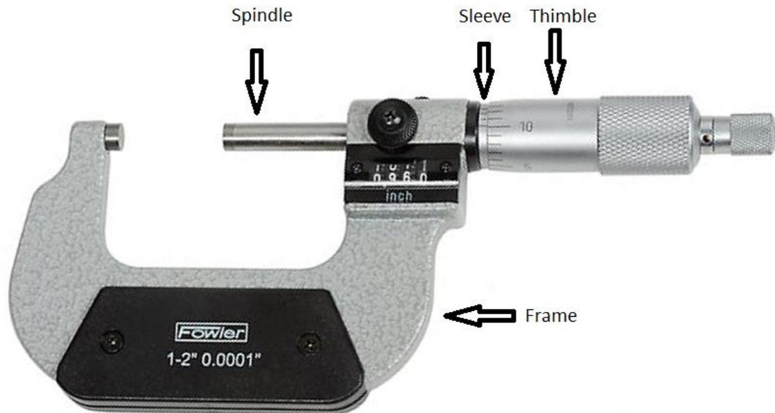
**Figure 4: The Fowler 1-2" digital micrometer.** The spindle remains in contact with the slide and enables measurement of the location of the moveable wire. The sleeve increases the precision of the micrometer to the ten thousandth of an inch. The thimble is rotated to move the spindle linearly. The frame fits into the slide casing which keeps it in a consistent location.
