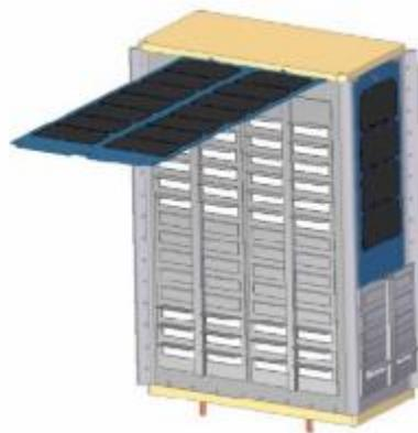
**Figure 14: Passive thermal louver** on NASA 6U CubeSat [13].
