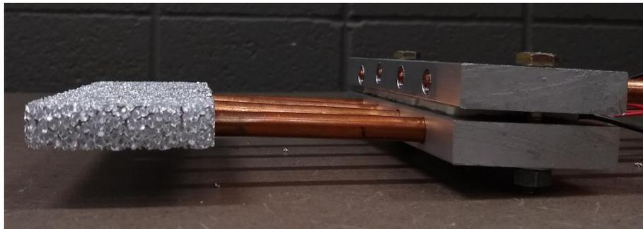
**Figure 5: Aluminum Foam Positioning.** The heat pipes are inserted into the aluminum foam block.
