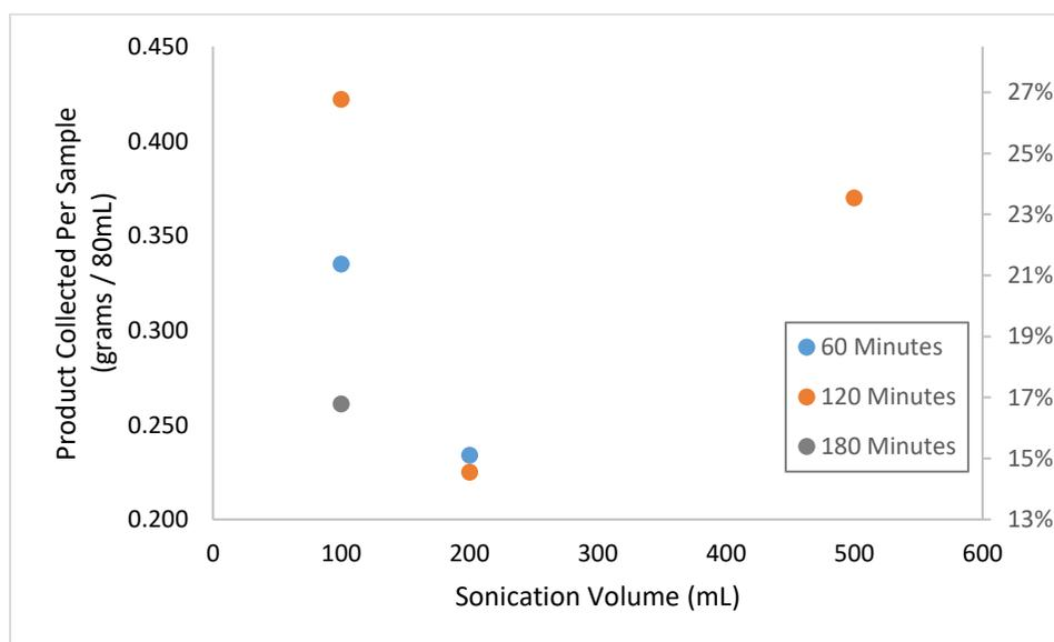
**Figure 1. Product collected per sample and percent yield by sonication volume.** The amount of product collected per sample is the raw measured dry weight. The percent yield was calculated using the beginning weight of graphite oxide used in each trial.
