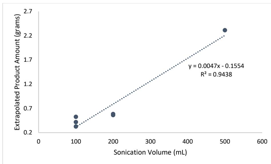
**Figure 5. Extrapolated product amount by sonication volume.** This graph shows the collected dry weight extrapolated out as though the entire sonication volume was centrifuged and dried. The approximately direct relationship between these values agrees with the previous conclusion that the overall production rate is unaffected by sonication volume.
