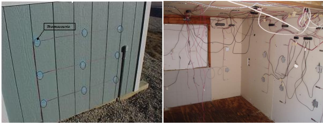
Figure 6: Outdoor (left) and indoor (right) sensor arrangement [26]
